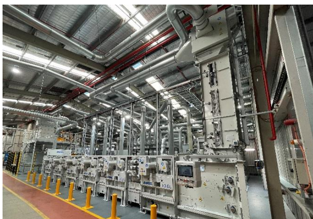
ANDRITZ reXline tearing for textile recycling at Sealy Australia's mattress plant in Brisbane
